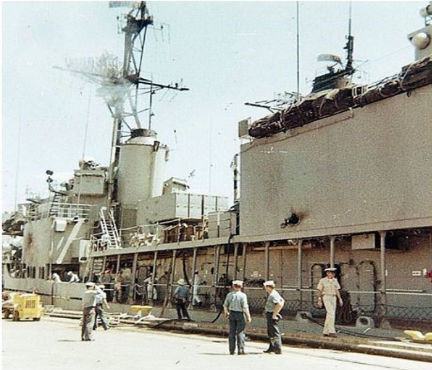
Damage sustained to the ASROC Magazine, 25 March 1967.
